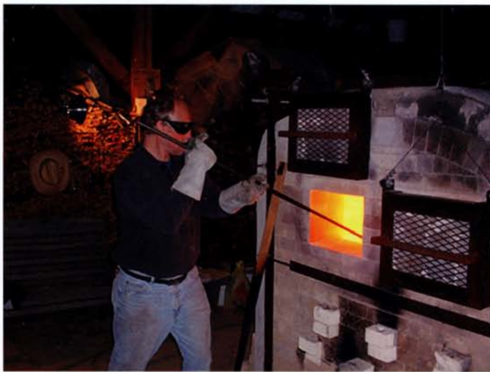
Tony Moore firing his anagama-Noborigama Kiln, using a long steel poker to knock down coals. Photo credit: Tom Loggia.
