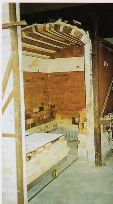
Top: Paul Chaleff's 10 m/long kiln with six side stoke ports each side. Above: Paul Chaleff's gas-fired car kiln used for large-scale sculpture
